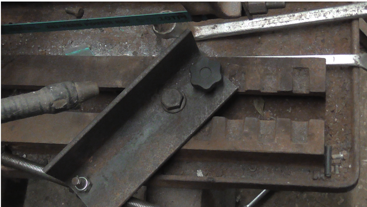
The finished clamp set for 45 degree cut.
