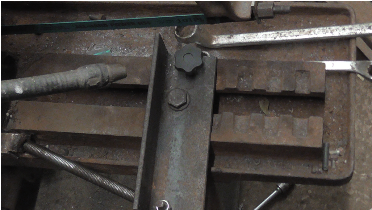
The finished clamp set for a right angle cut.
